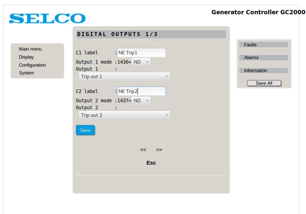
Figure 52 - Non essential consumer trip output setting
