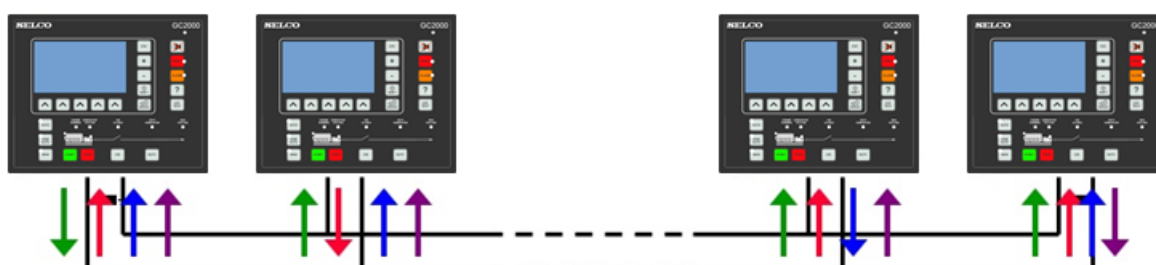
Figure 62 - Broadcasting data between multiple units
