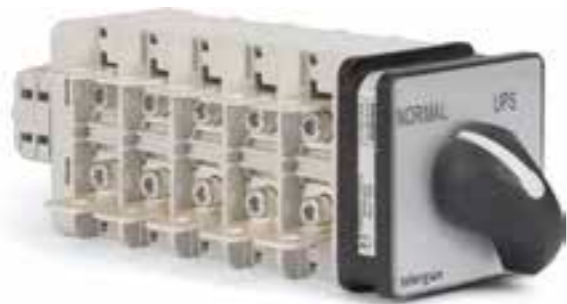
Cam switch T-175 for 200 A (approx. 100-120 kVA) Positions: NORMAL - UPS
