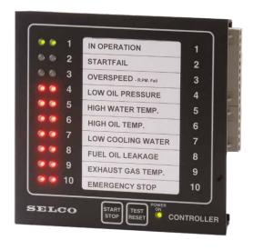
Start is obtained by activating the start input from a remote contact or by pushing the start button of the unit, if in manual mode. After a user configured delay the start will be initiated. It is possible to configure the unit to do up to 4 start attempts, with user configurable crank and rest periods.
