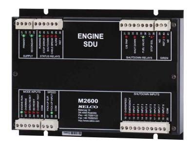
The unit furnishes 10 digital shut-down inputs. 1 is pre-defined for overspeed and another for emergency stop. All inputs are potential free dry contacts.
