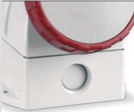
TOP version: threaded knockout hole inlets, version IP66/IP67, for quick fastening of the cable entry device. IP44 versions supplied with cable gland.
