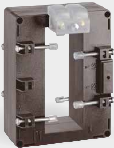
CT with cable/ passing bar (Primary currents: 40...8000A)
