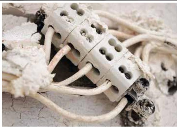
Even though the plastic enclosure has melted, the current is still flowing.
