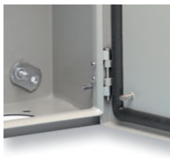
The enclosure has welded M8 bolts in the bottom of the base and M6 bolts in the door. There is also an M6 bolt for earthing on one side.
