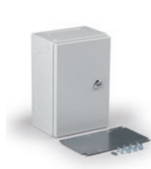
A 1.5 mm mounting plate complete with M8 bolts and earthing accessories are included in the delivery of standard enclosures.
