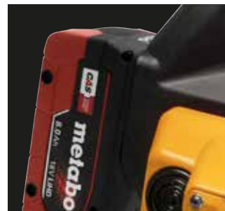
Automatic battery connection system
